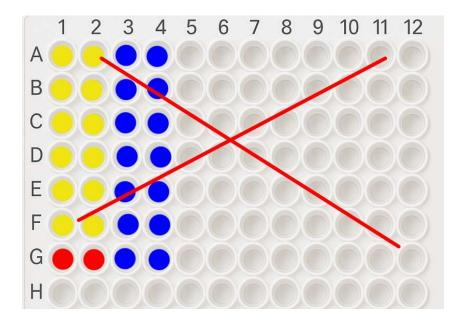
The image below is an incorrect example. (Data must start from the first column, i.e., cells A1, B1, C1, D1, E1, F1, G1, and H1 must contain values.)
