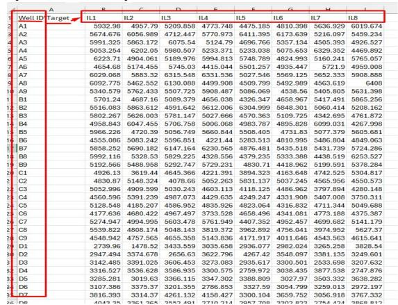
The first row of the CSV file is "Target Name". Please enter the correct target name for your test. The first column is "Well ID", and the valid range for Well IDs is from A1 to A12, B1 to B12, ..., up to H1 to H12. You may adjust the Well IDs according to your specific scenario. Make sure to fill in your standard (STD) and sample data using this template.
