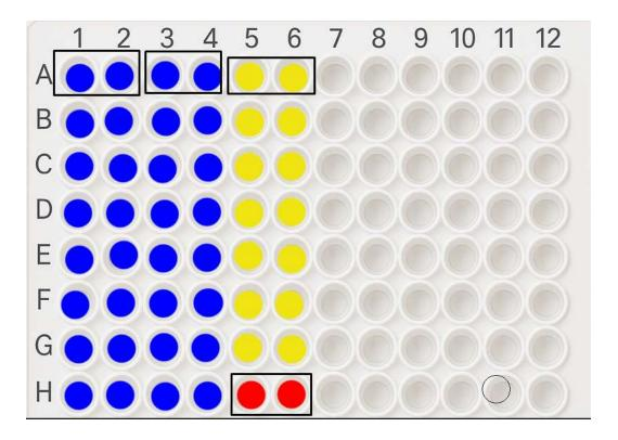
The image below shows two duplicate STD & NEG columns from Column 1 to Column 2, along with 32 samples. The CSV Well IDs range from A1-A10 to H1-H10
