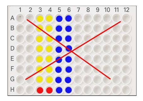
The image below is an incorrect example. (There should be no gaps between columns with data. For example, if columns 1 and 2 have values, column 3 must not be empty if column 4 or beyond contains data.)
